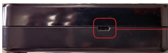
USB interface of debugger
